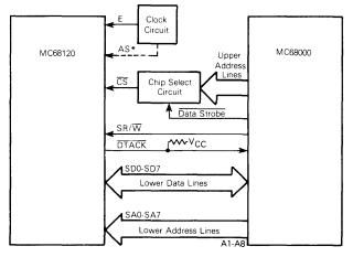
FIGURE 16 - ASYNCHRONOUS SYSTEM BUS INTERFACE
