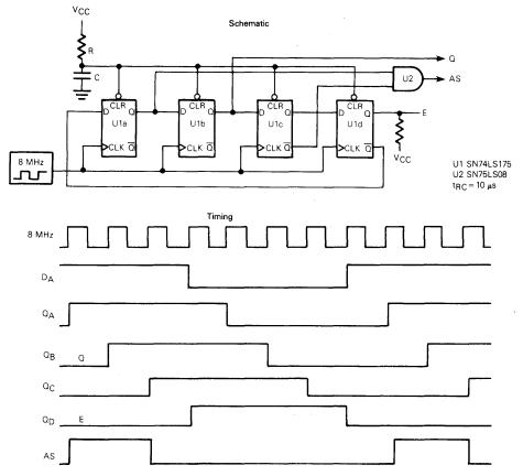
FIGURE 18 - CLOCK CIRCUIT EXAMPLE 1 - SCHEMATIC AND TIMING
