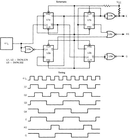
FIGURE 19 — CLOCK CIRCUIT EXAMPLE 2 — SCHEMATIC AND TIMING Schematic
