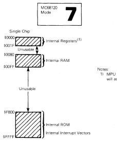
MPU reads of Port 3's Data Direction Register will access Port 3's Data Register instead.
