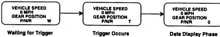
6. Once the trigger occurs, the **TECH 1** will continue to save data samples until its memory is full. The data display indicates that the trigger has occurred by replacing the flashing 'W' with a flashing 'T'. As soon as the memory is full, the data capture terminates automatically and the **TECH 1** goes to the Data Display phase.
