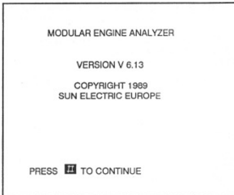
FIGURE 28. This is the first page the operator will see after the MEA-1500 SL is turned on.
